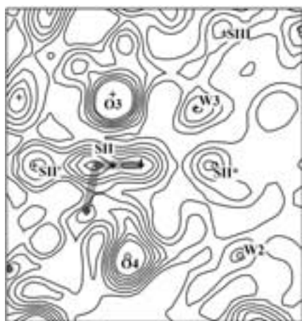
Figure 3. Observed electron density map (mapsize: 10 Å) before last-cycle refinement. Shown is a side-view of the six rings that containing the sulfite group (marked in grey). Water molecules are labeled W, cation sites are labeled SII and SII* according to their position. Electron density between framework oxygen O4 and oxygen atoms of the sulfite group suggest hydrogen bonding.
